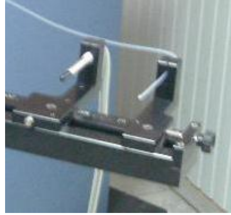
Two jigs for the in-air calibration of Ir-192 HDR and PDR sources
