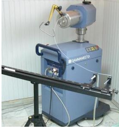
Two jigs for the in-air calibration of Ir-192 HDR and PDR sources
