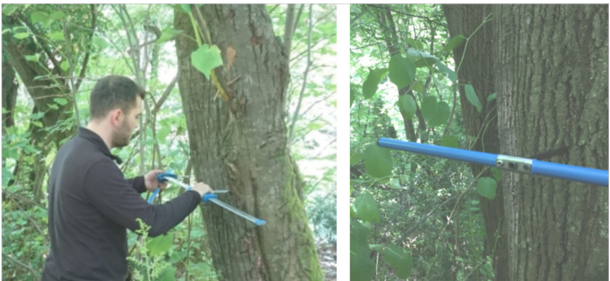
Figure 3. Diameter measurement (left) and trunk core sample collection (right) in the field
