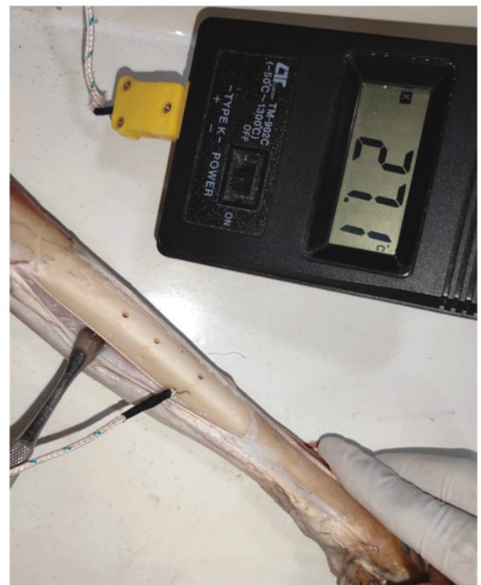
Figure 2. Temperature measurement with thermocouple thermometer.
